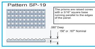
The raised conical prisms of pattern SP-19 give it a distinctive crystal like look similar to that found in injection molded panels. This pattern is also is highly efficient in reducing glare.
