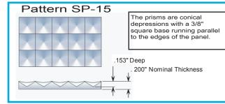
SP-15 panels are relatively rigid and sag resistant due to the thickness and the large female conical pattern. Panels up to 4'  $\times$  4' should be acceptable as far as sag is concerned. The conical pattern is highly efficient at diffusing light and reducing glare.
